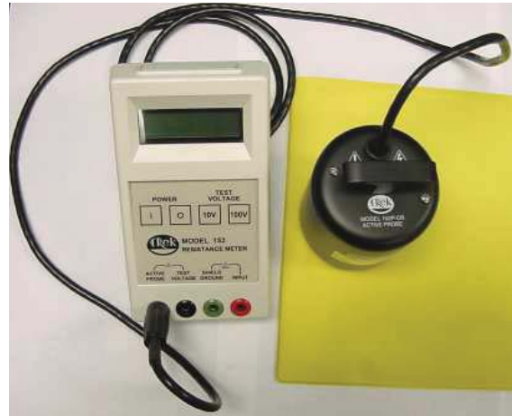
Figure 4: Surface resistivity measurement setup.
