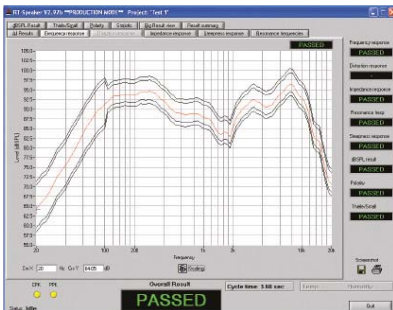
Frequency response measurement with absolute results
