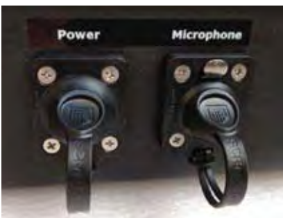
Waterproof connectors for microphone and external power supply (IP65 configuration)
