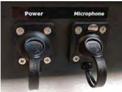
Waterproof connectors for microphone and external power supply (IP63 configuration)
