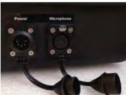
Removed protection plugs of waterproof connectors for microphone (IP63 configuration)
