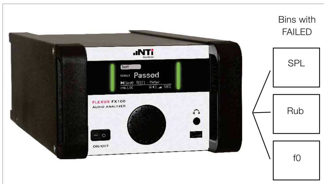
Automated splitting in FAILED production bins
