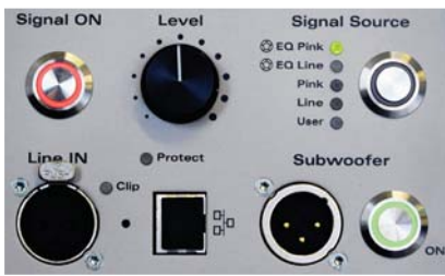
Control panel of PA3 Power Amplifier
