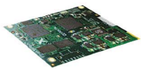
PHRXMDOLBY Dual Dolby decoder Dolby E/D/D Plus (mounted on CPU card)
