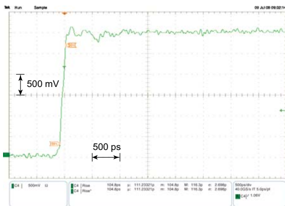
Fig. 3. TLP waveform measurement result at 40 GS/s [3]
