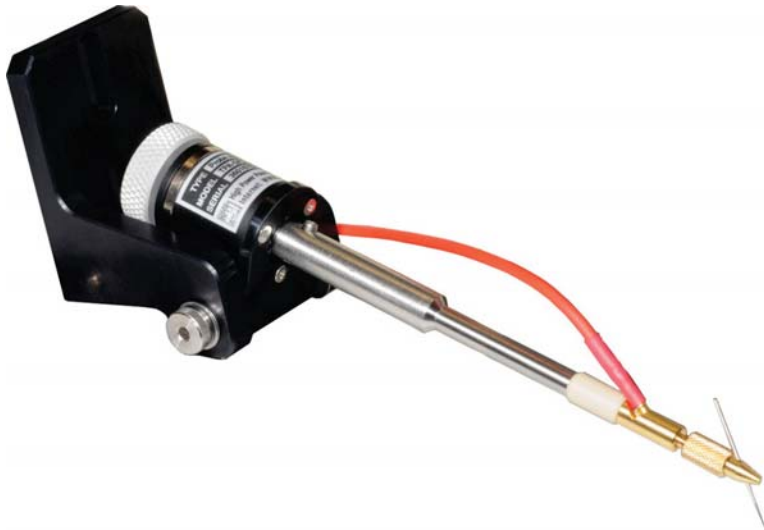
(a) TPA-GFG with separate cable connected to the contact pin
