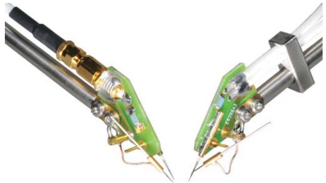
Figure 8: Detail view of the TPA-95 with GND needles connected.
