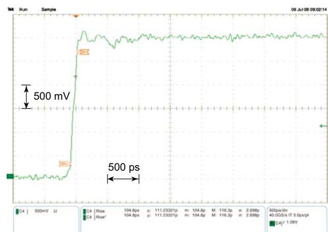
Figure 3: Typical output pulse waveform (40 GS/s)
