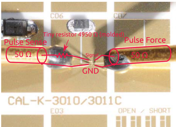
Figure 4: Fixed pitch picoprobes. Probing a reference device on the TLP calibration substrate. Detail view of Fig. 3 including equivalent circuit of the probe tips.
