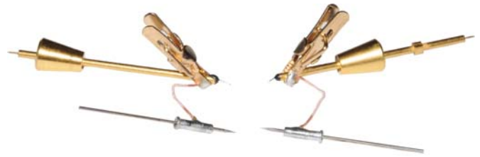
Figure 5: Ground fixture GF-A clamped on the probe tips
