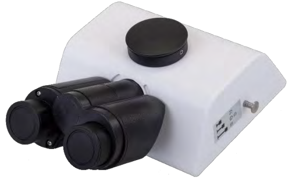
Viewing head with splitting ratio of 100:0 or 20:80 or 0:100 (eyepiece: trinocular) for BS-2078B
