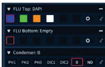
Fluorescence channel selection and observation mode control
