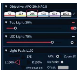
Objective magnification, light intensity and spectral control
