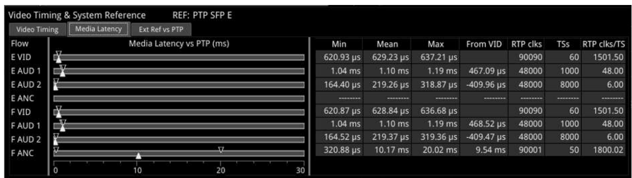
Figure 12-12: Media Latency Tab of the Video Timing & System Reference Instrument (ST 2110 IP Input)
