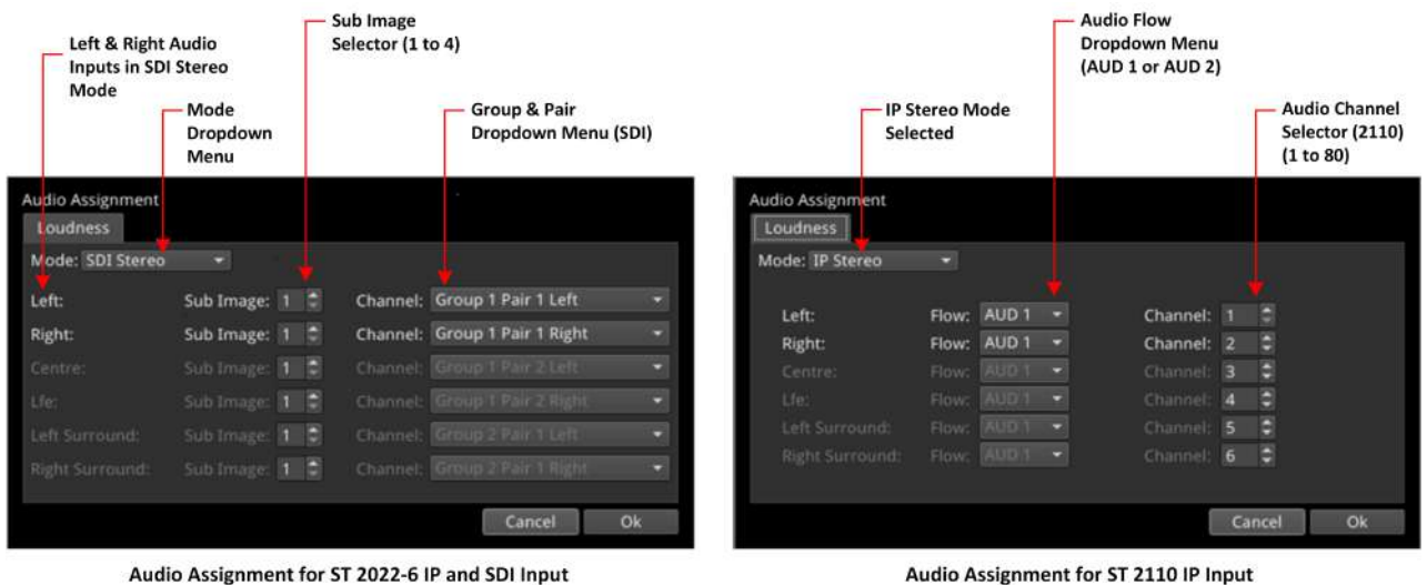
Figure 10-12: Audio Assignment for Loudness Input for ST 2022-6 IP / Optional SDI and ST 2110 IP Input
