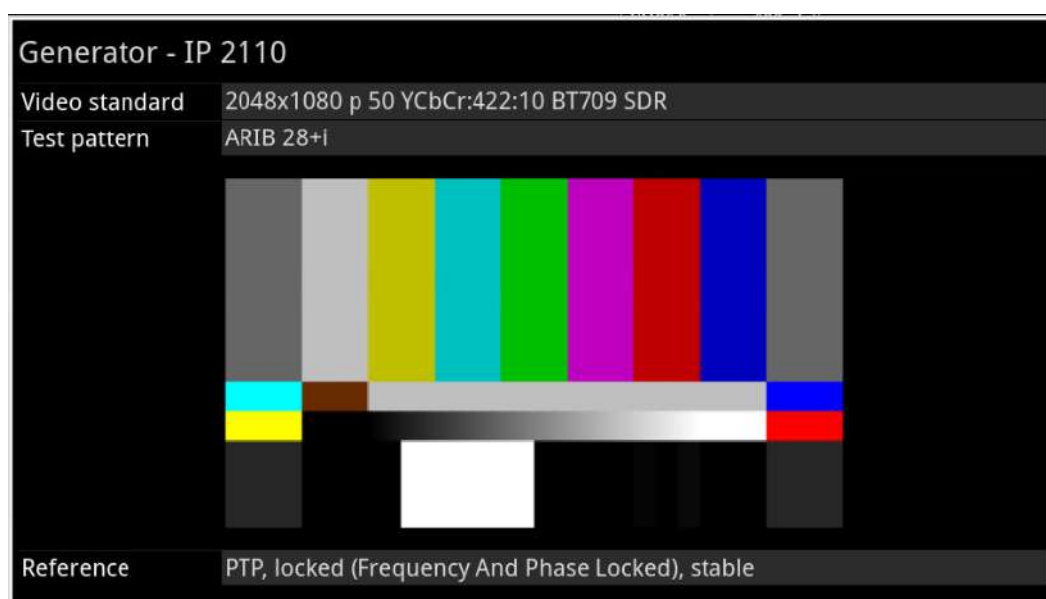
Figure 6-1: Generator Instrument (ST 2110 IP Output)
