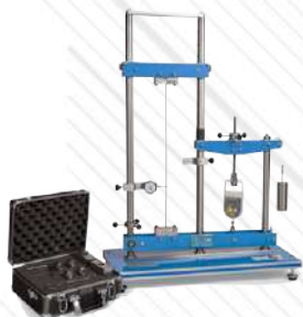
MEBM. Euler Buckling Modes Unit
