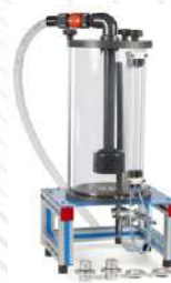
FME04. Orifice Discharge
