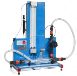
FME32. Static Pitot Tube
