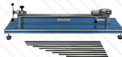
MTP. Torsion and Bend Unit
