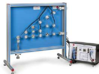
▶ MFCSI. Unit for studying Forces in Different Single Plane Trusses
