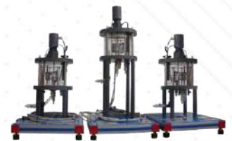
QRSC. Computer Controlled Stirred Tank Reactors in Series for QRC
