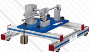
MEMT-4. Rolling Friction in Wheels
