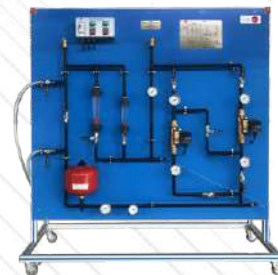
▶ TPVST. Pressure Vessel and Safety Features Training Unit
