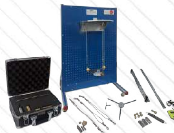
MSHU. Simple Harmonic Motion Unit
