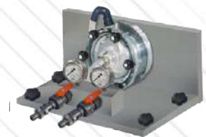
MDU-SSCP. Set to Study Cavitation in Pumps
