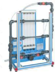
FME23. Basic Pipe Network Unit
