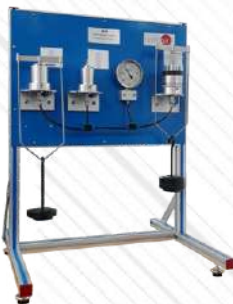
▶ MSH. Simple Hydraulic Unit
