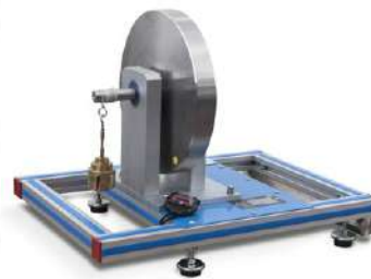
MIF. Inertia Flywheel Unit
