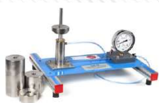
FME10. Dead Weight Calibrator
