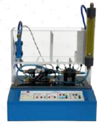
BS4. Flow Test Module
