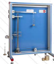
▶ MCD. Thin Cylinder Unit
