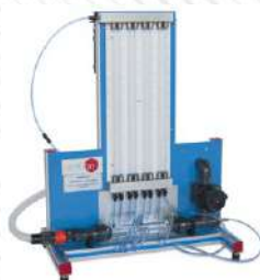
FME03. Bernoulli's Theorem Demonstration
