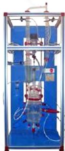
QRQA/D . Isothermal Reactor with Stirrer and Distillation
