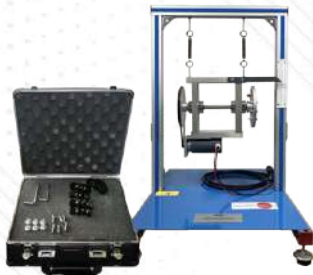
MES. Simple Balancing Unit
