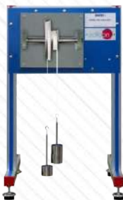
MELH. Unit for studying Hooke's Law
