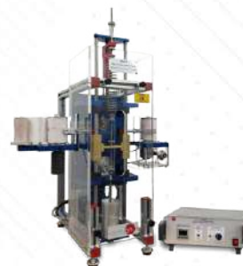
MVLF. Free & Forced Vibration Unit
