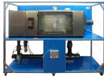
HFCC. Computer Controlled Flow of Compressible Fluids Unit
