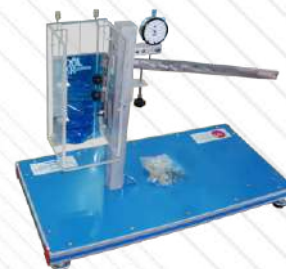
▶ EEFCR. Creep Testing Unit
