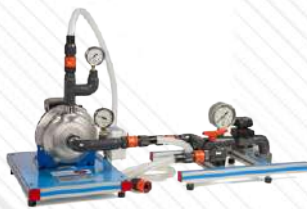
FME12. Series/Parallel Pumps
