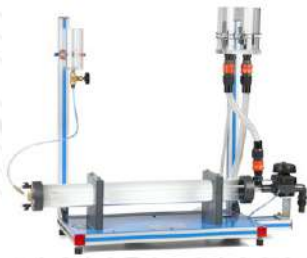
FME31. Horizontal Osborne Reynolds Demonstration
