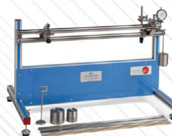
MTP. Torsion and Bend Unit
