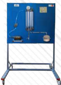
▶ TEVT. Expansion Vessel Training Unit
