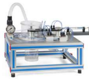
FME27. Axial Flow Turbine
