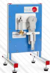
▶ MEX. Cam and Follower Mechanism
