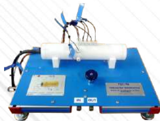
TXC/ER. Radiation Errors in Temperature Measurement Module for TSTCC
