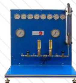
TPT. Nozzle Pressure Distribution Unit
