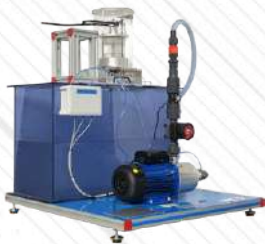
HT-K. Kaplan Turbine Model
