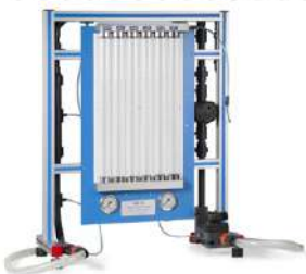
FME05. Energy Losses in Bends
