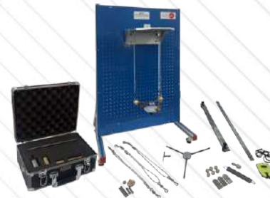
MSHU. Simple Harmonic Motion Unit
