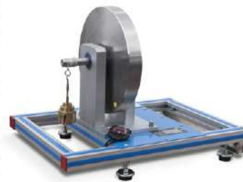
MIF. Inertia Flywheel Unit
