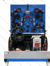
TBM/G. Comprehensive Gasoline Test and Diagnostic Bench for Combustion Engines with Fault Simulation
