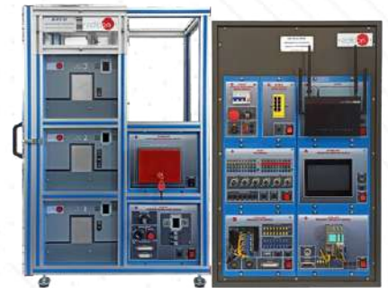
AE-PLC-SE. Elevator Control Application.
