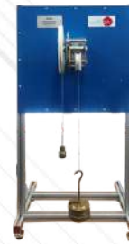
▶ MMEL. Winch Mechanism
