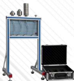
MEBM. Euler Buckling Modes Unit
