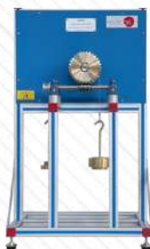
▶ MSDA. Simple Drives Assembly Unit
