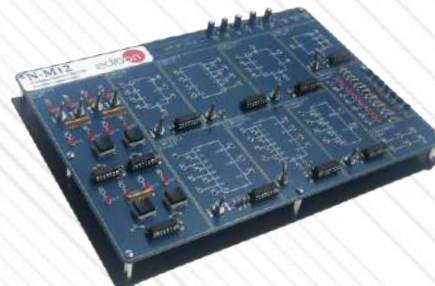
N-M12. Basic Combinational Circuits Module.
