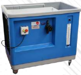
FME00. Hydraulics Bench
