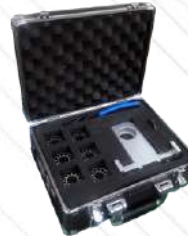
MDU-SRBF. Set of Roller Bearings with Faults
