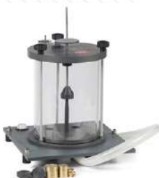
FME01. Jet Impact on Surfaces
