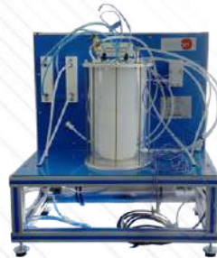
QRFT . Tubular Flow Reactor
